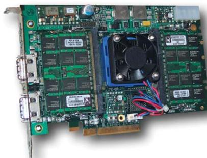
A pair of 10-gigabit Ethernet ports (CX4) provide an impressive 20Gbps of network I/O. An optional mezzanine expansion board further increases flexibility by supporting additional I/O options, such as 10G optical interfaces or multiple 1G ports. The TILExpress-20G card is also available as a PCIe-based co-processor solution with no I/O interfaces for computation-only applications.
