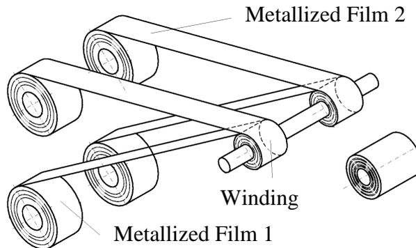
An alternative production process for film capacitors is the so called **stacked** technology [4]. This is done by winding big wheels of metallized film that is latter cut in smaller capacitors. At the end, one obtains a series of hundreds capacitors in parallel, which make this technology extremely appropriate for pulse applications, but inappropriate for power applications.
