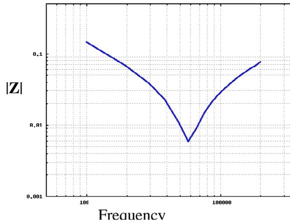
Figure 36. Impedance versus frequency for the 110 µF, 450 V<sub>R</sub> capacitor
