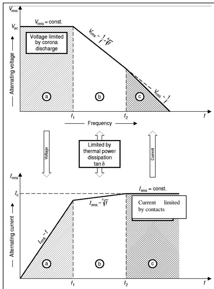
Figure 22. Alternating voltage and alternating current load limits
