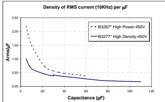
Figure 32. Comparative of maximum admissible  $I_{rms}$  current for existing EPCOS High Power and the new High Density DC-link design
