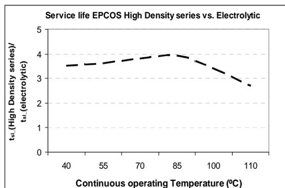
Figure 34. Comparison of the service life ( $t_{50}$ ) of our new High Density series with a typical electrolytic capacitor for power applications [14]
