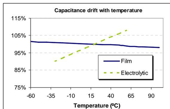
Figure 29. Comparison of capacitance drifts of Electrolytic and Film technologies [4]
