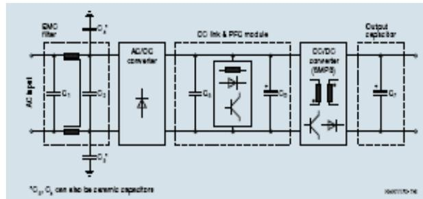
Figure 27. SMPS modules are typical industrial applications where DC-Link capacitors play an important role
