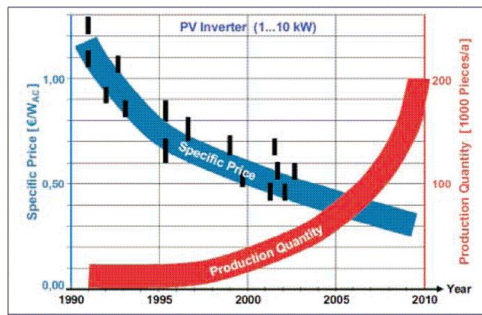
Figure 40. Development and prognoses of specific cost and production quantity for different range of PV inverters [22].
