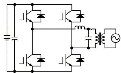
Figure 4. Traditional design of buck inverter with an electrolytic DC-link capacitor.
