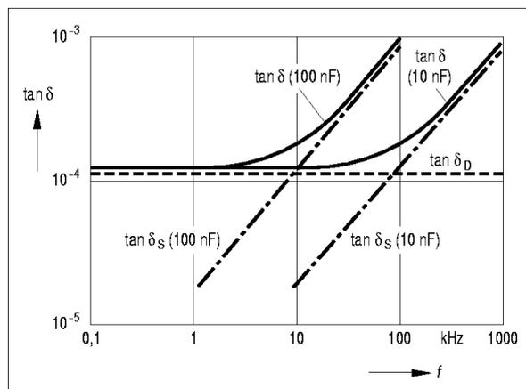
Figure 16. Dissipation factor versus measuring frequency (schematic representation using two polypropylene capacitors of different capacitance as examples).
