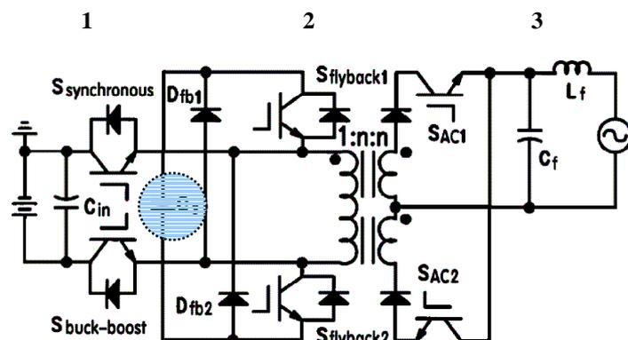
Figure 6. Innovative topology of solar inverter with a small intermediate DC-link film capacitor ( $C_s$ ).
