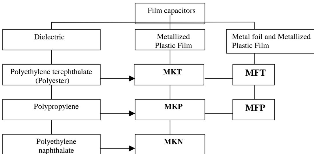
Figure 7 Classification of film capacitors according to DIN 41 379
