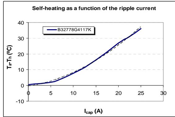
**Figure 31. Dependence of the increment of temperature due to dissipation losses in the B32778G4117K (450 V<sub>R</sub>, 110 μF) capacitor. Dashed line depicts a second order polynomial.**
