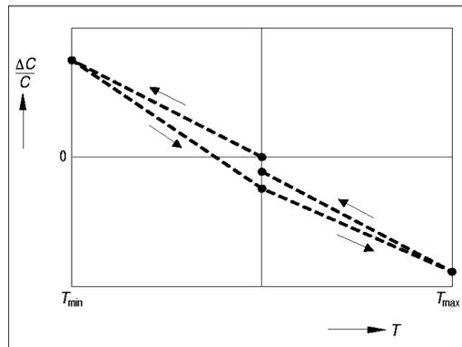
Figure 12. Capacitance change versus temperature (schematic curve)
