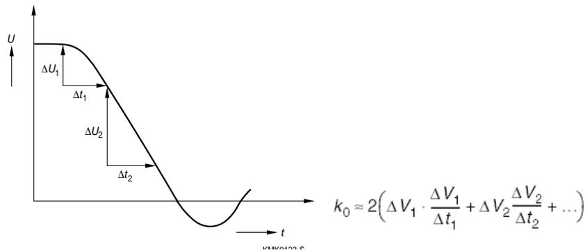
Figure 24. Piece-wise linear approximation of a voltage pulse
