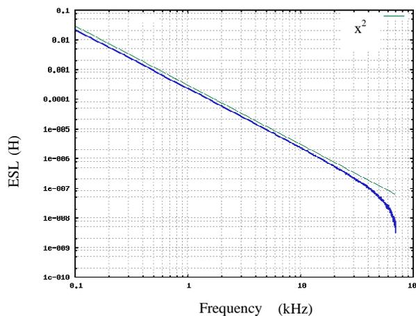
Figure 37. Measurement of the ESL for the 110 µF capacitor. For comparison, an  $x^2$  potential law has also been plotted (thin line).
