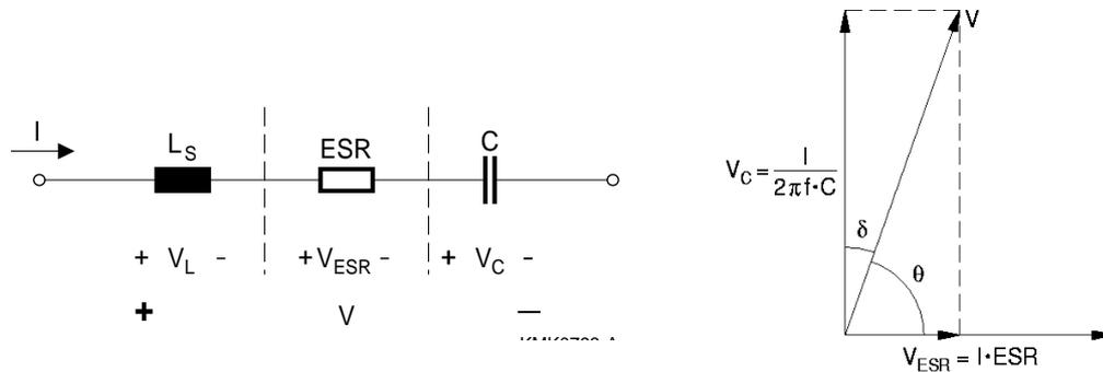
Figure 15. Simplified capacitor model for AC. Complex voltage calculation.
