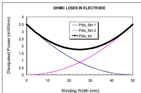
Figure 30. Simulation result of the dissipated power (P) due to ohmic losses in the film capacitor and contribution from each of the electrodes.
