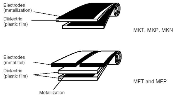
**Figure 8 Examples of typical film and foil arrangements**
