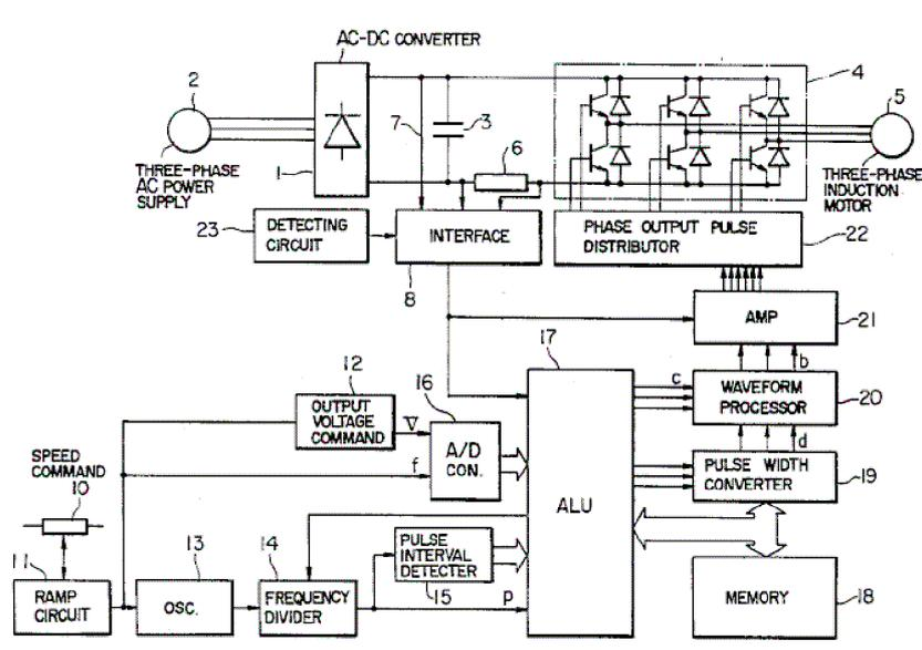
Figure 2. Block diagram showing a general arrangements of a PWM DC-AC inverter system according to [28]
