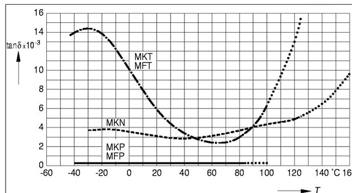
Figure 18. Dissipation factor  $\tan\delta$  versus temperature T for  $f = 1$  kHz (typical values)
