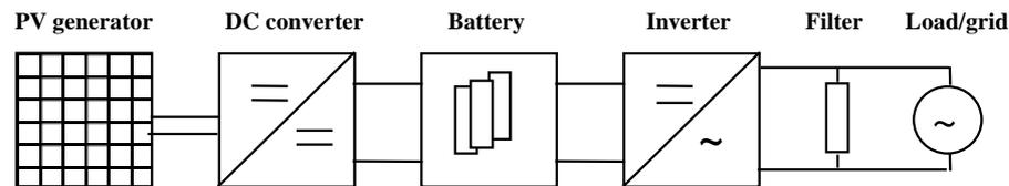
Figure 1. Block diagram of a general PV system
