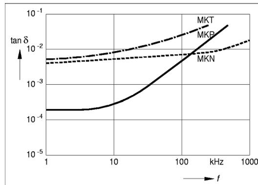
Figure 17. Frequency dependence of the dissipation factor, e.g. for  $C_R = 0.10 \mu\text{F}$  (typical behaviour)
