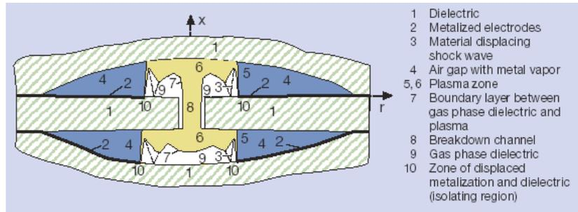
**Figure 25. Schematic of the self-healing area during electrical breakdown**
