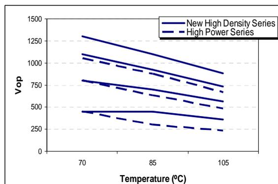
Figure 33. Continuous operation voltages for the high power and the High Density series
