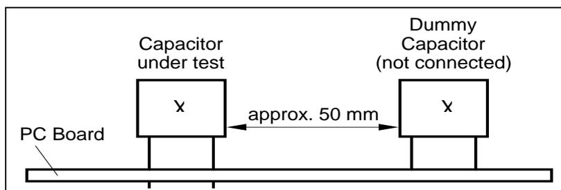
Figure 23. Test fixture to measure the self-heating under working conditions.
