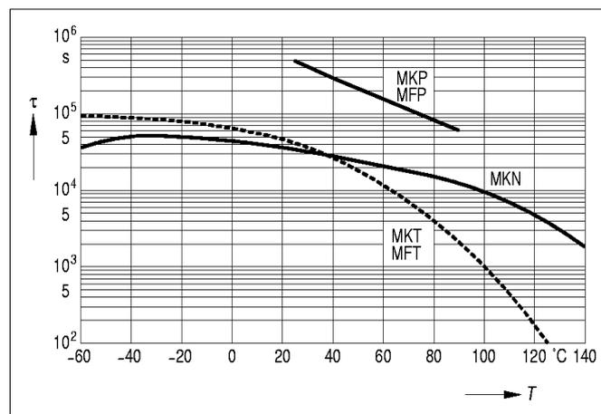
Figure 19. Insulation as self-discharge time constant  $\tau (= R_{is} \times C_R)$  in s ( $= \text{M}\Omega \times \mu\text{F}$ ) versus temperature T (typical values)
