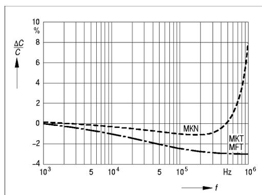
Figure 14. Relative capacitance change  $\Delta C/C$  versus frequency (typical example)
