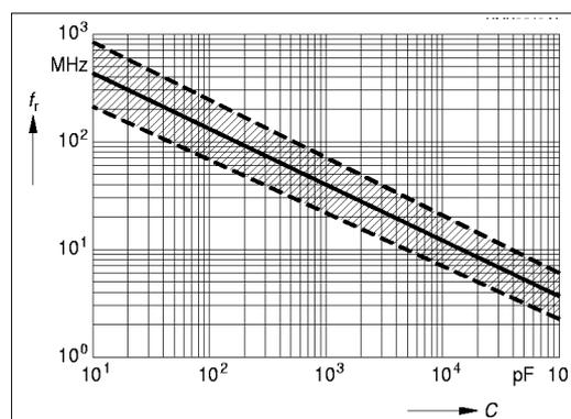
Figure 20. Resonant frequency versus capacitance (typical values)
