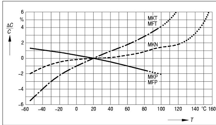
Figure 11. Relative capacitance change  $\Delta C/C$  versus temperature  $T$  (typical values)
