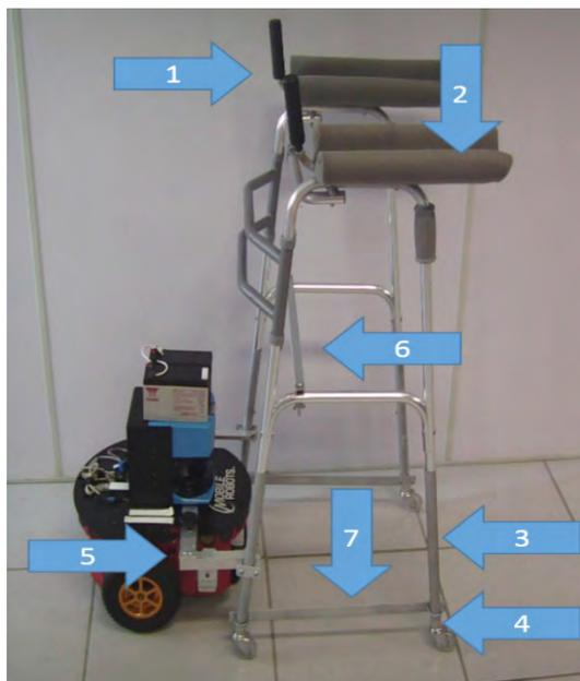
Figure 5. Robot adaptation to work as a walker.
