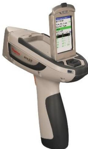
Figura 11: XRF portable Niton XL3t (*Thermo Scientific™*).
