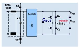
Figure 28. Basic scheme of an induction hob circuit.
