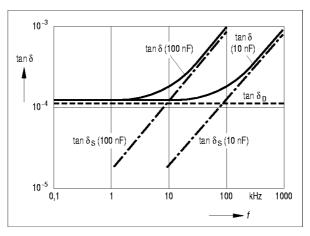
Figure 16. Dissipation factor versus measuring frequency (schematic representation using two polypropylene capacitors of different capacitance as examples).
