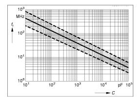
Figure 20. Resonant frequency versus capacitance (typical values)
