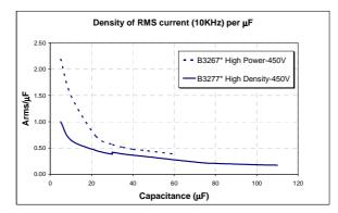
Figure 32. Comparative of maximum admissible I<sub>rms</sub> current for existing EPCOS High Power and the new High Density DC-link design
