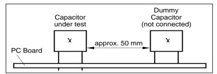
Figure 23. Test fixture to measure the self-heating under working conditions.
