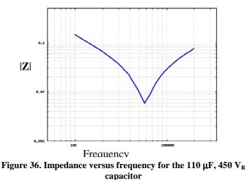
Impedance, ESR, and ESL values and maximum admissible  $I_{rms}$  are also defined for those capacitors, giving to converter designers the basic information to select the right product according to their needs. Figure 37 shows the impedance behaviour with frequency for the representative 110  $\mu$ F capacitor.
