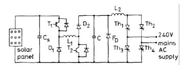
Figure 5. Novel configuration for grid connected solar photovoltaic inverter [7].
