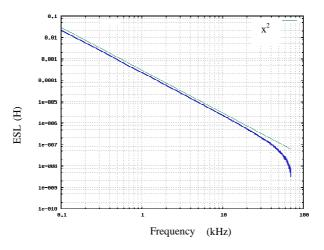
Figure 37. Measurement of the ESL for the 110 µF capacitor. For comparison, an x<sup>-2</sup> potential law has also been plotted (thin line).
