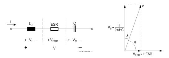
Figure 15. Simplified capacitor model for AC. Complex voltage calculation.
