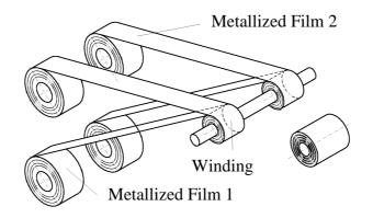
An alternative production process for film capacitors is the so called **stacked** technology [4]. This is done by winding big wheels of metallized film that is latter cut in smaller capacitors. At the end, one obtains a series of hundreds capacitors in parallel, which make this technology extremely appropriate for pulse applications, but inappropriate for power applications.
