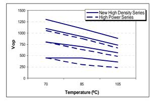
Figure 33. Continuous operation voltages for the high power and the High Density series
