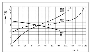
Figure 11. Relative capacitance change  $\Delta C/C$  versus temperature T (typical values)
