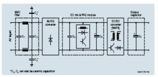
Figure 27. SMPS modules are typical industrial applications where DC-Link capacitors play an important role
