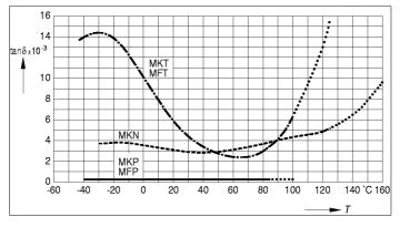
Figure 18. Dissipation factor  $tan\delta$  versus temperature T for f = 1 kHz (typical values)
