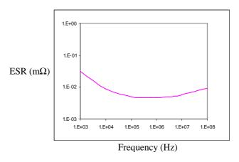
Figure 17. ESR versus Frequency for a MKT capacitor.
