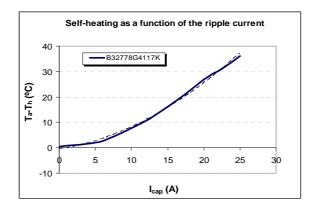
Figure 31. Dependence of the increment of temperature due to dissipation losses in the B32778G4117K (450  $V_R$ , 110  $\mu$ F) capacitor. Dashed line depicts a second order polynomial.
