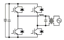
Figure 4. Traditional design of buck inverter with an electrolytic DC-link capacitor.
