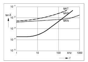
Figure 17. Frequency dependence of the dissipation factor, e.g. for  $C_R = 0.10 \ \mu F$  (typical behaviour)
