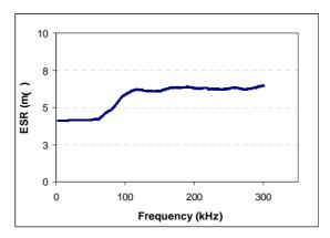
Figure 38. Typical ESR measurement for the 110  $\mu F$  capacitor.
