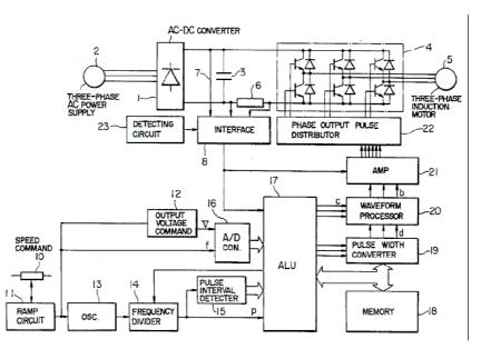
Figure 2. Block diagram showning a general arrangemets of a PWM DC-AC inverter system according to [28]
