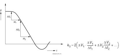
Figure 24. Piece-wise linear approximation of a voltage pulse
