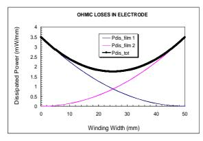
Figure 30. Simulation result of the dissipated power (P) due to ohmic losses in the film capacitor and contribution from each of the electrodes.
