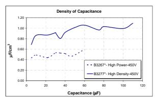
Figure 35. Maximum capacitance range reached with the new design rules of the new high Density series.
