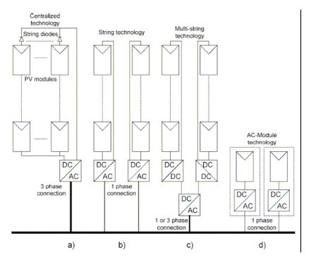
Figure 3. Historical evolution of PV generator designs, going from the classical centralised technology to the most modern AC-modules. Figure taken from [19].
