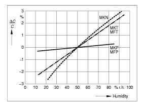
Figure 13. Relative capacitance change  $\Delta C/C$  versus relative humidity (typical values)
