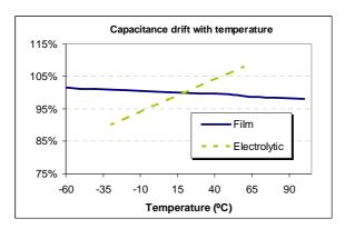
Figure 29. Comparison of capacitance drifts of Electrolytic and Film technologies [4]
