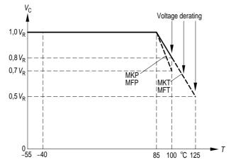
Figure 21. Maximum permissible continuous voltage in relation to ambient temperature.
