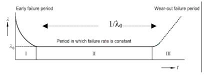
Figure 41. Typical failure rate curve of a product.
