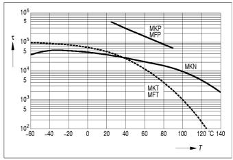
Figure 19. Insulation as self-discharge time constant  $\tau$  (=  $R_{is}~x~C_R)$  in s (=  $M\Omega~x~\mu F)$  versus temperature T (typical values)
