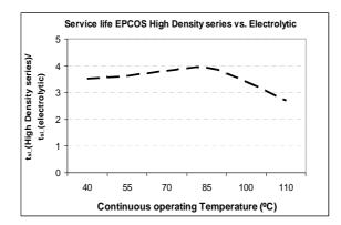
Figure 34. Comparison of the service life ( $t_{sl}$ ) of our new High Density series with a typical electrolytic capacitor for power applications [14]
