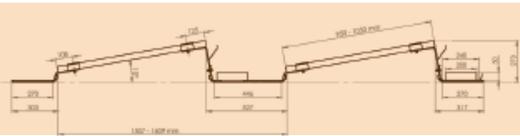
LEICHTmount 2.0 S 10° with a shading calculation area of 18°/527mm row spacing
